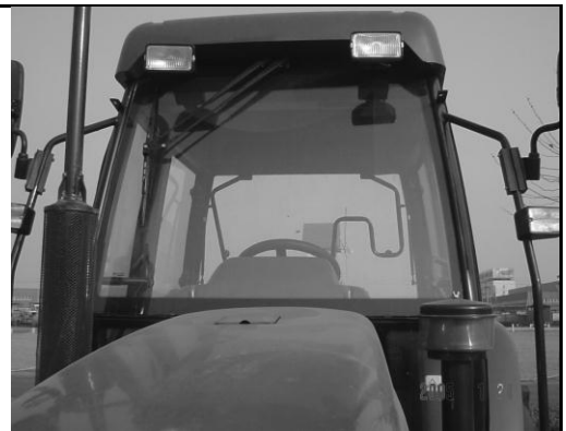
Figure 2-43 Roof (Work) Lights
