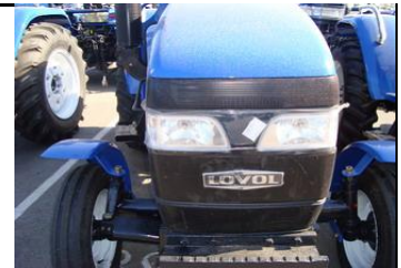
Figure 4-14 Combined Front Head Lamp Position
